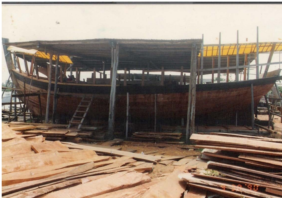
Figure 276. Brazilian boat shed used to construct a replica caravel. Courtesy of Morgan Sanger.
